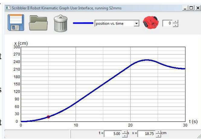
*Illustration 3: A position vs. time graph that matches the velocity vs. time graph in illustration 2. When started simultaneously, robots programmed with the two graphs run side-by-side to within millimeters. The red dot highlights the midpoint of the first segment, which can be dragged (or set by entering values) to curve the segment. A parabola is drawn between the two endpoints and the midpoint.*
