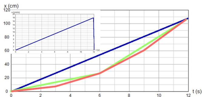
*Illustration 4: Successive approximations to an accelerated motion (velocity graph inset) are programmed using a position vs. time graph with one (blue), two (green), and four (red), constant velocity segments, and tested by racing them against the accelerating robot. By six segments (not shown), the motions are barely distinguishable and students can envision that the limiting sequence will end with a smooth curve.*
