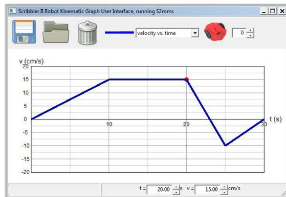
*Illustration 2: After drawing a kinematic graph, the student clicks on the red robot icon to send the program to the robot. The red dot highlights the currently selected point, which can be edited by dragging it or by entering values in the text box in the bottom status bar.*
