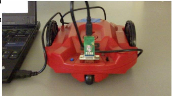
*Illustration 1: A USB-serial adapter and USB cable are used to connect the robot to the computer.*
